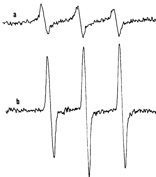
Figure 3 - ESR spectra of MLV-insulin loaded with Tempocholine (gain : 5.10^5 ). Insulin is covalently coupled to the outer surface of these liposomes -a- before lysis -b- after chemical lysis
